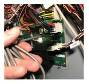
3. If the cable does not reach the site controller, you will need to extend it with a CAT-5 cable or a straight through Male-Female DB9 serial cable.
