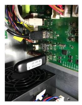
2. Be sure you are using the current CFINIT, version CFINIT117.2.5 In the 4.1 logic box, the CFINIT must be placed in one of the top two USB ports as shown above.
