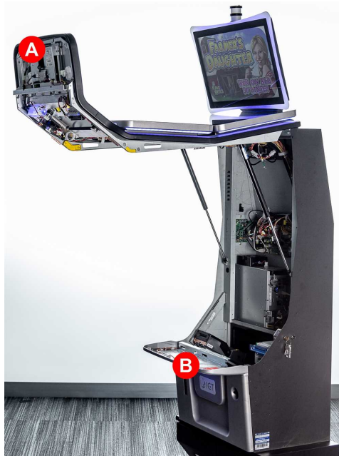
Figure 1-9 Main Door Open
