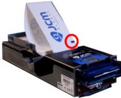
Figure 2-27 FutureLogic GEN5, Loading Paper
