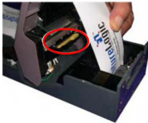
Figure 2-28 FutureLogic GEN5, Clearing Paper Jam
